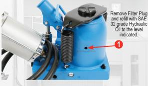
Regularly lubricate the Air motor and Manual Pump Pivots.
